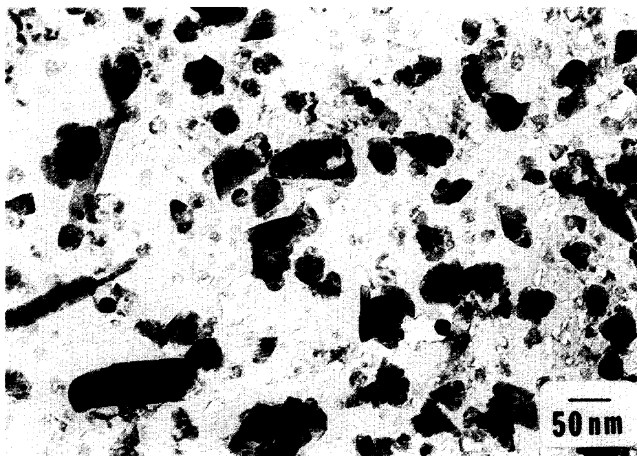
FIG. 8. \text{Fe}/\text{Al}_2\text{O}_3 specimen after heating in \text{CH}_4 for 20 h continuously at 700^\circ\text{C} , following heating in \text{H}_2 for 10 h (5 h at 500^\circ\text{C} and 5 h at 700^\circ\text{C} ).
